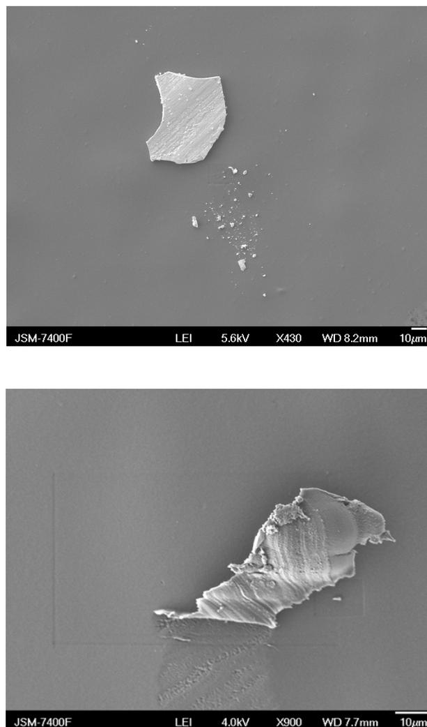
Figure 4.12: The disintegration of HNPs after 72 h.
