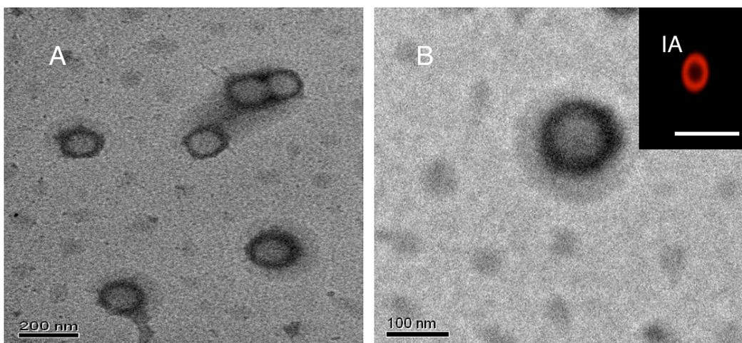
Figure 4.3 The TEM images of HNPs without inner core. Inset image IA is obtained by confocal microscopy.
