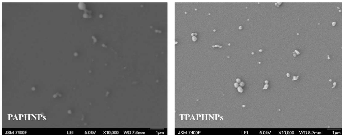
Figure 5.5 SEM images of functionalized siRNA encapsulated PLGA hollow nanoparticles
