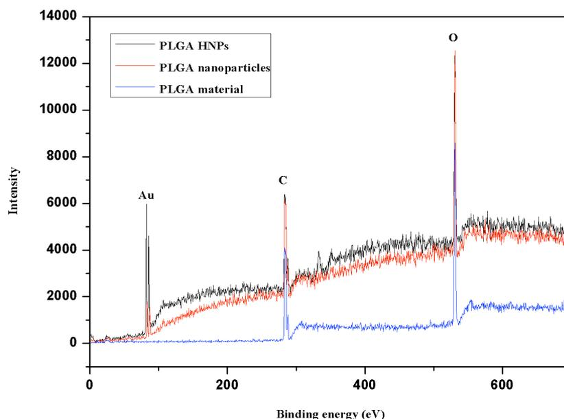
Figure 4.7 XPS spectra of NPs. XPS spectra of PLGA, PLGA HNPs and PLGA NPs and peaks showing presence of carbon and oxygen (Au from the substrate)
