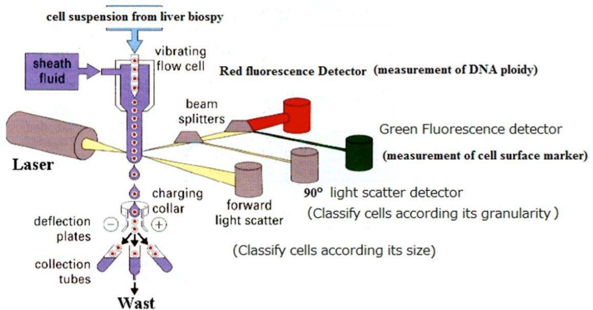
Figure 2.3. Flow cytometry working principle
