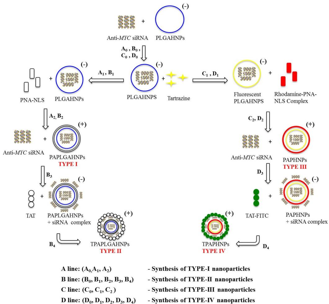
Figure 5.1: Schematic representation of synthesis of four types of anti-myc-siRNA encapsulated PLGA NPs: Type 1- PAPLGAHNPs, Type 2- TPAPLGAHNPs (non-fluorescent NPs), Type 3- PAPHNPs and Type 4- TPAPHNPs (fluorescent NPs).
