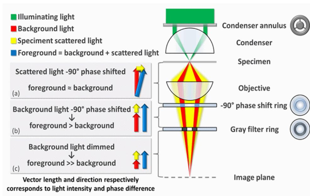
Figure 2.2: Principle of phase contrast microscopy
