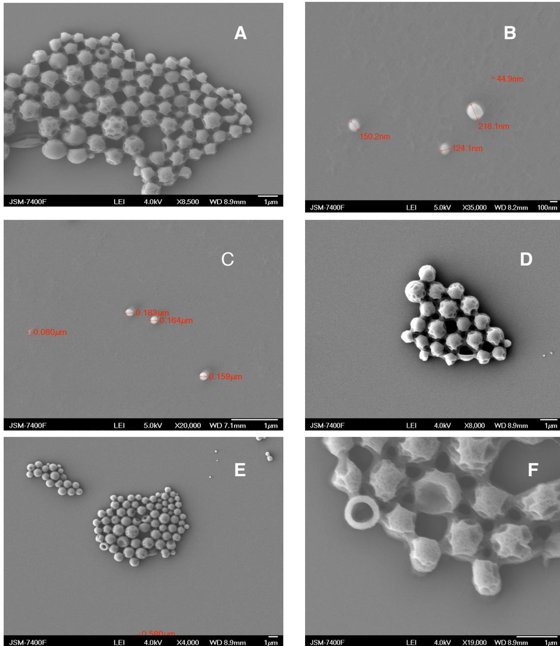
Figure 4.2 The SEM images of HNPs at various magnifications.
