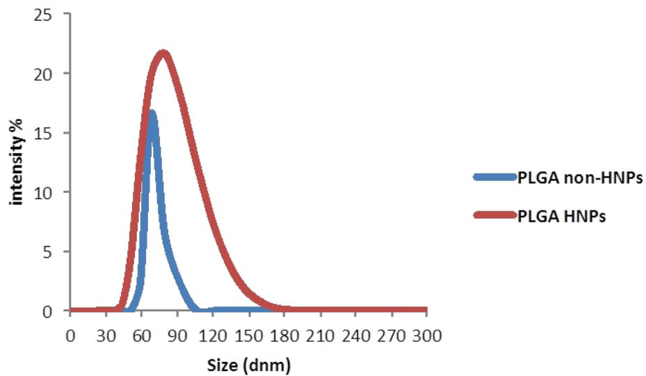
Figure 4.5 Particle size distributions of HNP and non-HNP PLGA NPs.
