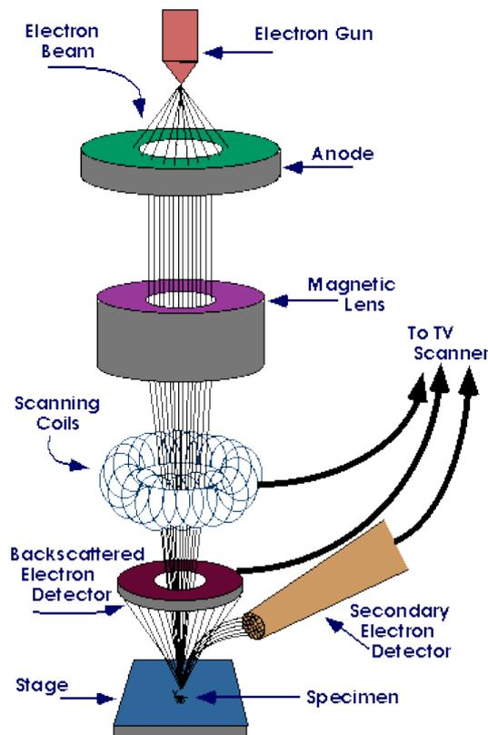
Figure 2.1 Working principle of SEM to detect the morphology of specimen
