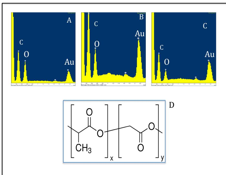
Figure 4.6 The EDS analysis graph for commercially obtained PLGA (A). (B) and (C) show the EDS of HNPs and non-HNPs with presence of oxygen and carbon.(Au is from substrate) (D) Structure of PLGA.
