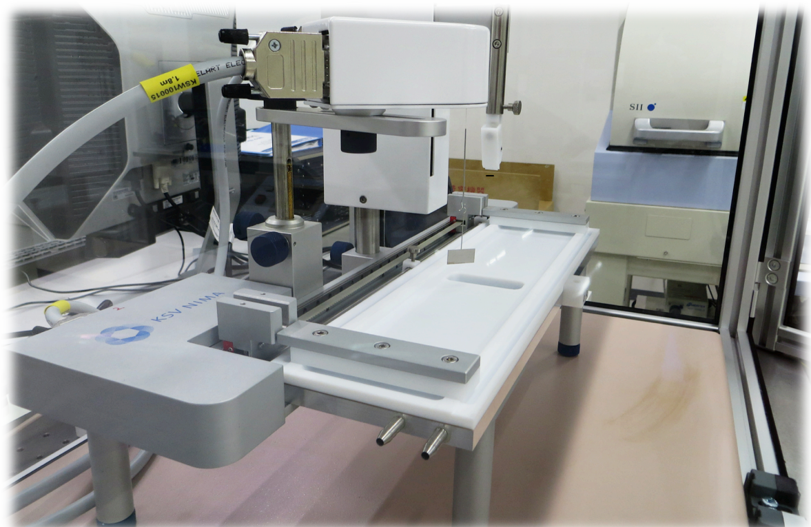
Figure 4. KVS–NIMA LB Trough was used for the present work. Monolayer assemble and SP-area isotherm of GO were measured using this setup, the trough top inner dimensions of medium size LB were measured as 364 mm × 75 mm × 4 mm, SP was monitored using tensiometer attached to a wilhelmy plate.
