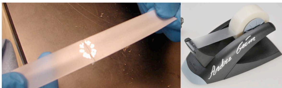
Figure 12. Micromechanical exfoliation of graphite flake. Adhesive scotch tape is pressed against a 2D crystal so that the top few layers are attached to the tape. The tape with crystals of layered material is pressed against a surface of choice. Upon peeling off, the bottom layer is left on the substrate.
