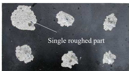
r_{cr}=0.1 Depth:Middle, \sigma_0=0.48\text{N/mm}^2 , c\sigma_B :Low level (a) CH-M10LL-cy
