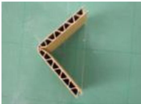
Fig. 3-9 Geometric shape of corner parts in corrugated fiberboard<sup>44)</sup>
