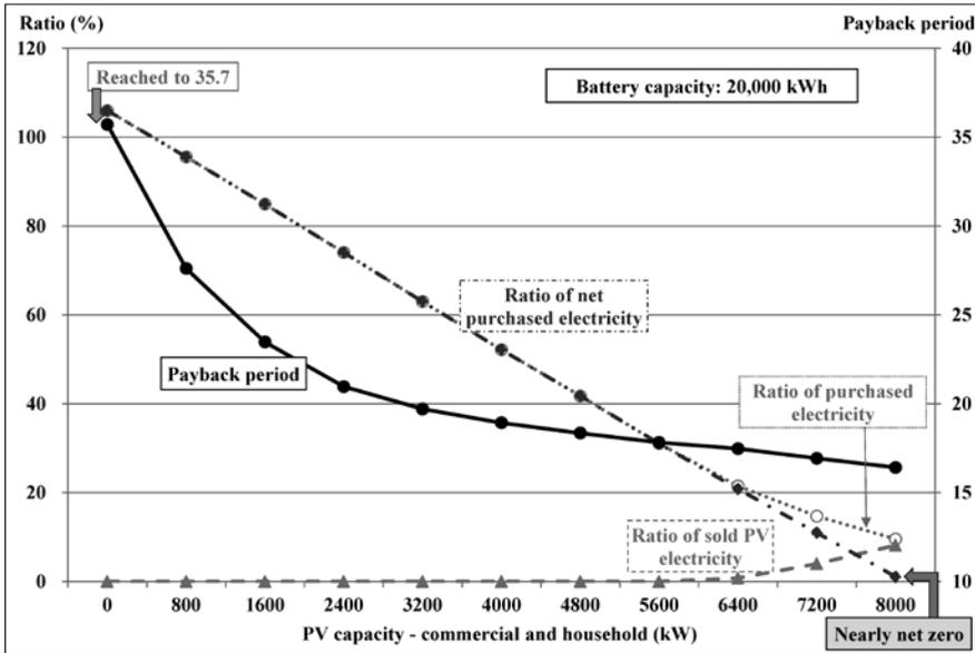
Fig. 9 Changes in cost and performance by with varied commercial and household PV capacity (battery capacity fixed at 20,000 kWh)
