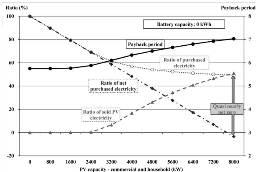
Fig. 10 Changes in cost and performance with varied commercial and household PV capacity (no battery, 0 kWh)
