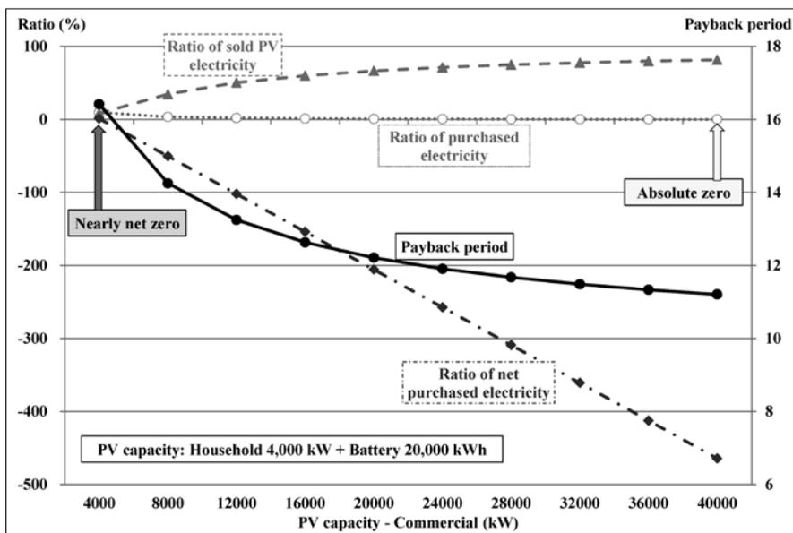
Fig. 8 Changes in cost and performance with varied commercial PV capacity (household PV capacity fixed at 4,000 kW and battery capacity at 20,000 kWh)
