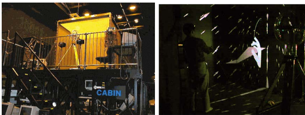
Figure 1. CABIN. Left: overview of CABIN, which has five screens, namely top, bottom, front, left and right. Right: flow field visualized in CABIN. Arrows indicate flow velocity vectors.
