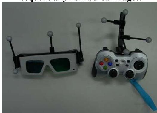
Figure 5. The controller and the stereo glasses. Four balls attached to the controller and the glasses are the markers for a visual motion capture system.
